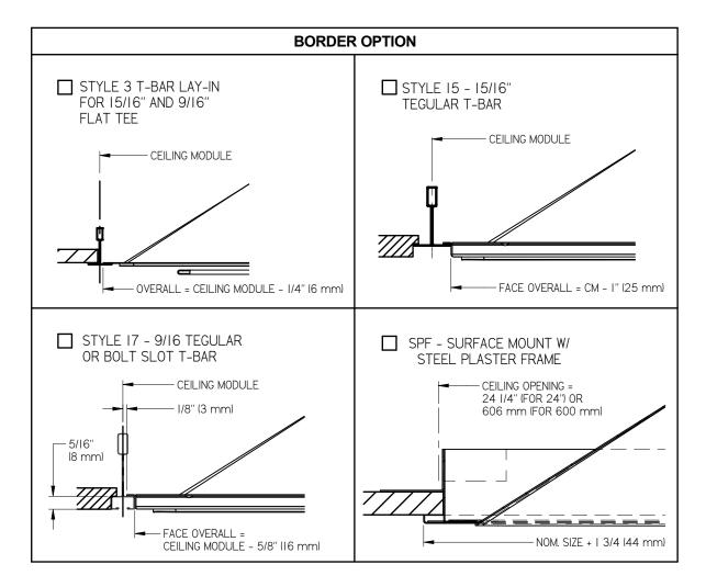
NOTE - METRIC DIMENSIONS HAVE BEEN ROUNDED TO THE NEAREST MILLIMETER
