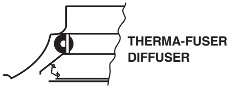
FIG. 7 FIELD INSTALLED FOAM BAFFLE ▼
