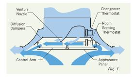
80°F/26.5°C. Changeover back to cooling is completed when the supply air temperature reaches 68°F/20°C.
