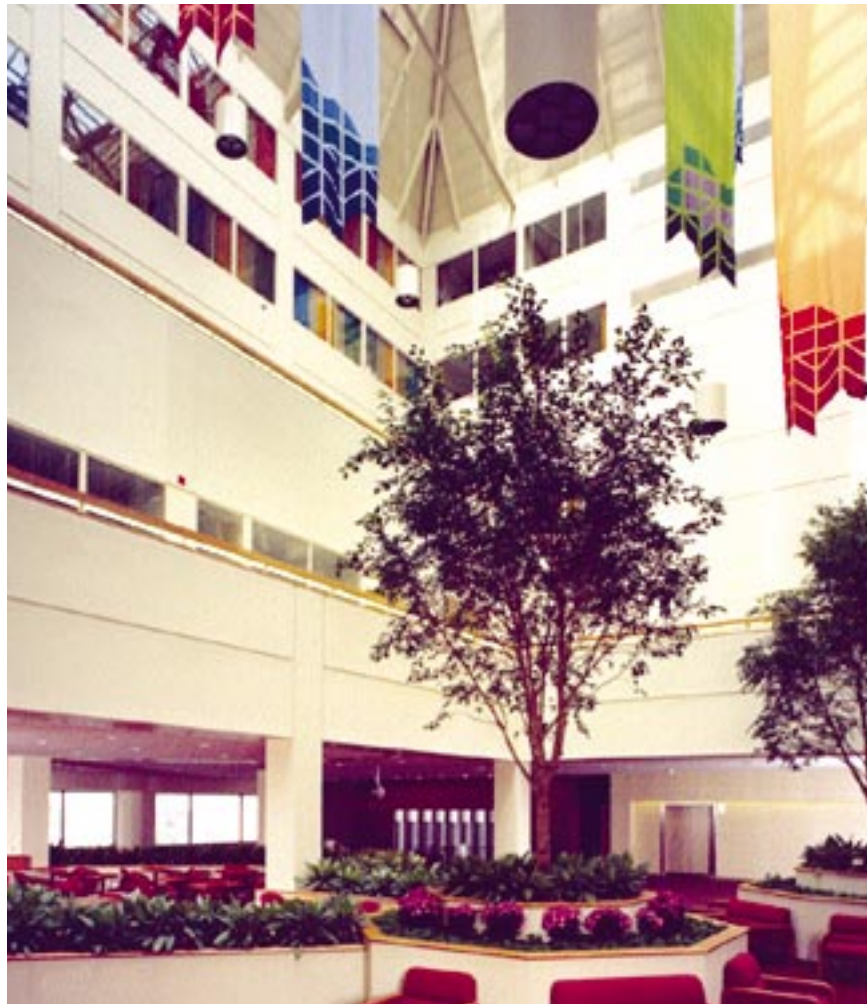
Although an atrium can present its own set of design issues due to height and possible smoke migration, the contents of this atrium illustrate a light-hazard condition.
