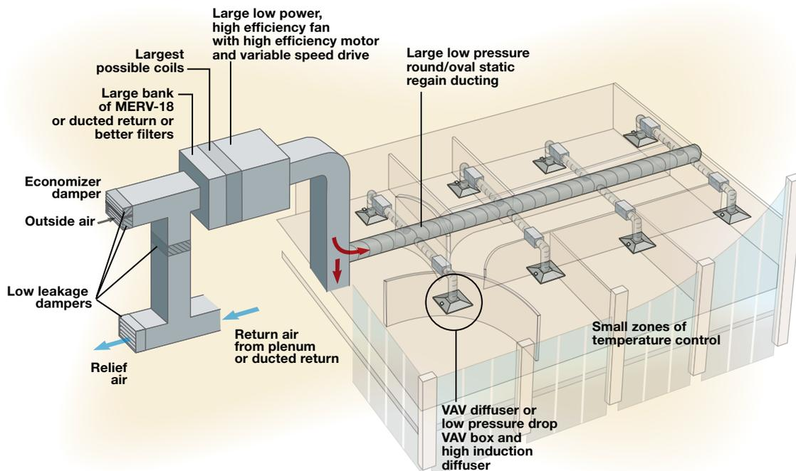
Figure 2: A ducted high performance air system
